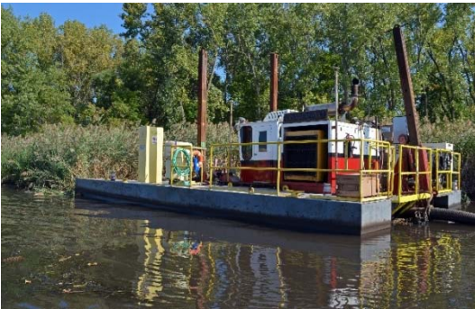
Figure 3: 8-inch Hydraulic Dredge
